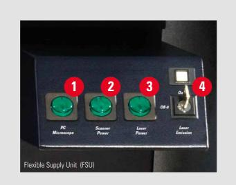
For system configuration with FSU: Turn on the power supply for the PC **1**, the scanner **2** and the lasers **3** by pushing the green buttons and turn the laser key 4, to open the laser shutter.
