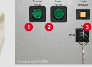
For system configuration with CSU:  $\rightarrow$ Turn on the PC and await the booting process. Then turn on the power supply for the scanner **1** and the lasers **2** by pushing the green buttons and turn the laser key 3, to open the laser shutter.
