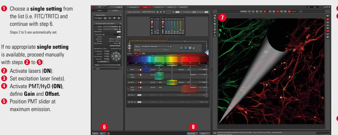
6 Start Live scan\*. **1** Click **QLUT** to switch to Glow. Change **Z Position** by turning the respective wheel on the control panel until you get the brightest signal (focal plane).
